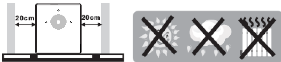
Figure 1. Placing of the UPS
